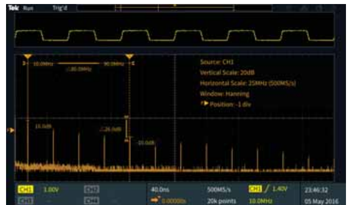
The time domain source waveform can be displayed above the FFT frequency spectrum.
