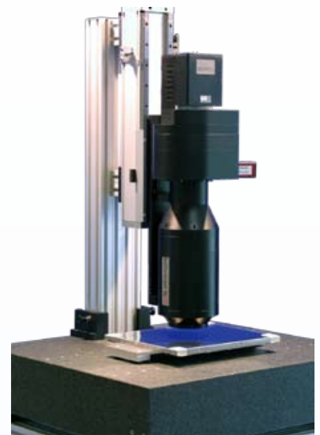
Laboratory bench with motorized Z axis
