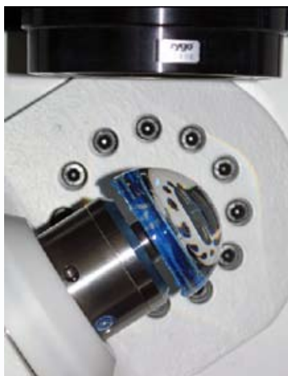
First hemispheric lens during QA by stitching interferometry
